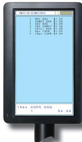
Rotate the screen for three portrait configurations. The SAM4s ML700 automatically senses portrait mode.
