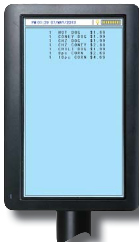
Rotate the screen for three portrait configurations. The SAM4s ML700 automatically senses portrait mode.
